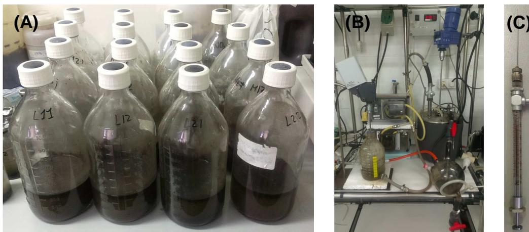
Schema and image of non-continuous (A) and discontinuous (B) experiment set-ups (C) Syringe for taking biogas sample
